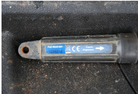
A temperature measuring and recording device (a logger)
